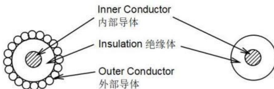
Fig.1 Cross section of coaxial 图1. 同轴线截面图
